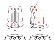
**STABILITY TESTS FRONT TILTING** Load: 27 kg Applied in the furthest point of the seat from the rotation axis
